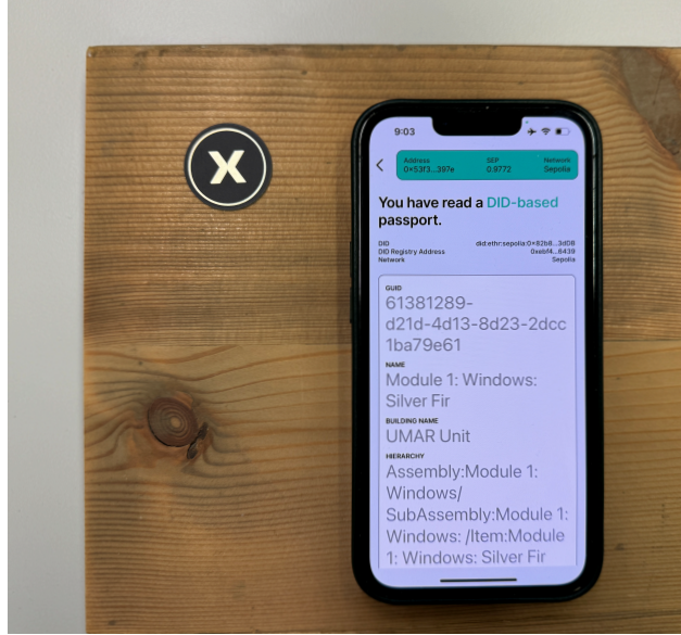
Figure 7: Image of the application after reading the HaLo data carrier (left) attached to a wooden component
